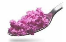
**Spectral data:** Excitation is best performed at 552 nm and fluorescence measured at 576 nm.
