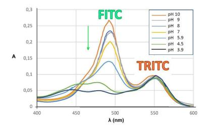
Fig. 2 UV-Vis spectra depicting the dependence of two visible features of FTD upon varying pH
