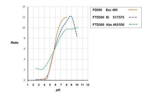
Fig. 3 pH-dependence on the ratios of emission and absorbance of FTD500 and those of a singlefluorophore involving dextran analogue (FITC-Dextran) of equal MW (FD500)
